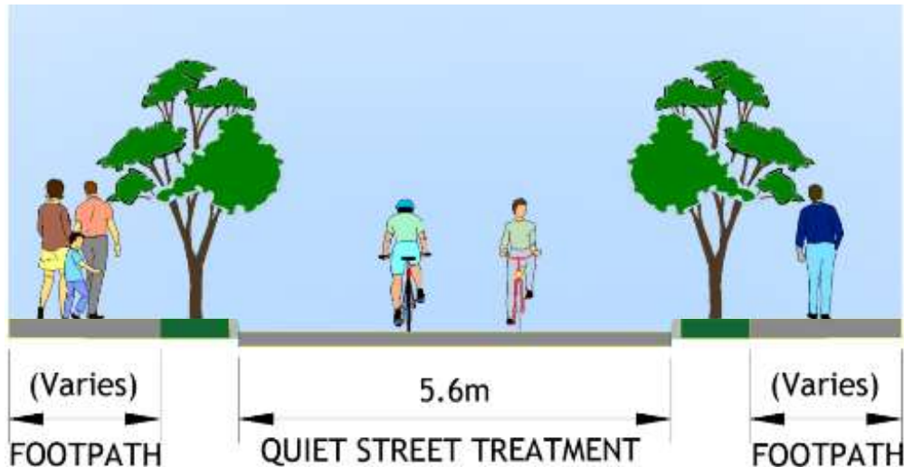
Figure 6.58: Route Option BK1 Cross-Section C-C
